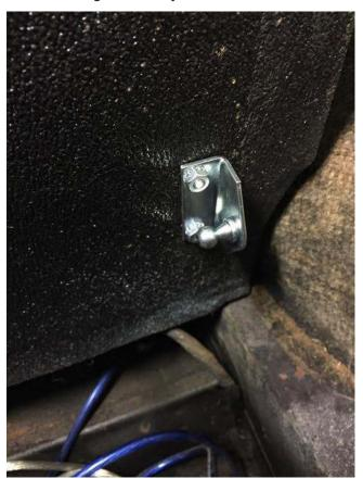
7. Snap on the Strut, then close and open the access panel to ensure everything operates smoothly. If you need to remove the Strut, simply put a small flat blade screwdriver under the black locking spring at the end of the Strut, and pull the Strut free.
