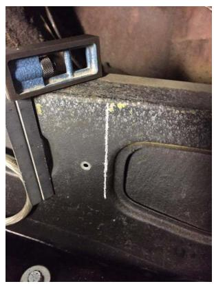
2. Measure down 5/8 inch to find your drill point. Countersink this location, and accurately drill a small hole. Now enlarge this small hole with a 5/16 inch bit, so that you then can attach the Ball Stud.
