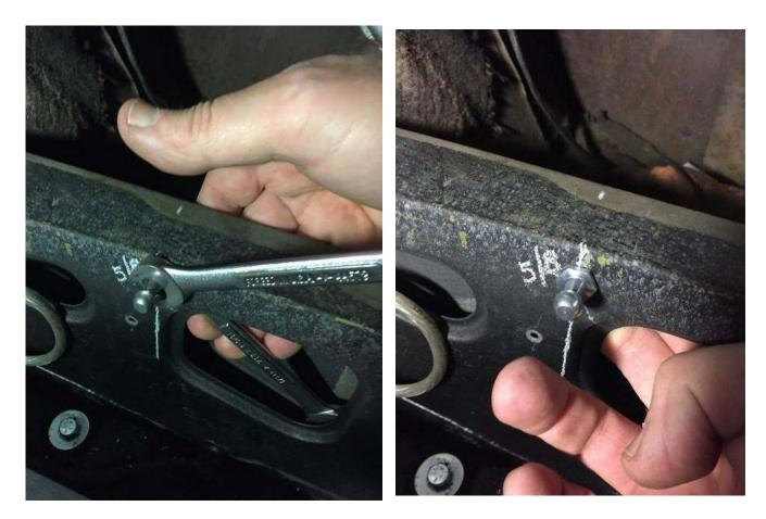
3. Close your access panel, and measure to the top bracket location as shown. Start by drawing a line parallel to the edge of the panel, off-set by 2.5 inches.
