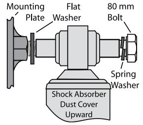
Attach the bottom ends of the shock absorbers by passing an M12 X 60 mm bolt through a large flat washer, the loop of a shock absorber, the lower shock link bracket and a second flat washer. Use a nyloc nut, finger tight at first, to secure the assembly.
