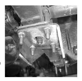
**TIP**: On some vehicles, the exhaust pipe will limit the clearance necessary for the 60 mm bolt to be inserted through the shock absorber bottom eye and into the left bracket (see page 6). If this seems likely, loosely attach the bottom eye of the left shock absorber before proceeding to the next step.
