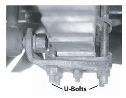
The rubber pads that fit over and under the leaf spring deteriorate with age and can be the cause of knocking noises and a hard ride. New pads are inexpensive and worthwhile installing while the U-Bolts are removed.
